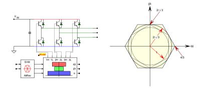
A Two-Level Inverter is mostly enough for controlling the current inside the electric machine
