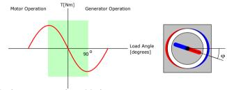
Maximum power when angular displacement  $= \Phi = 90$  degrees Is it a motor or is it a generator?
