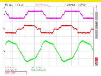
Lower trace, leakage inductor current (lpp=1.0 Ampere), and bridge output voltages(Vpp=48v), of the DAB with phase difference of 45 degrees, operating at 100kHz, Vdc=24v.
