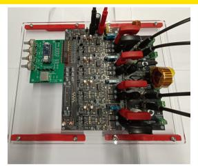
Low voltage hardware trainer, where switching frequency, duty cycles and phase shift can be manually changed by the student during operation of the DAB. Voltages across and current through the transformer can be measured with the coaxial cables.
