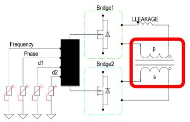
Principle schematic of the low voltage hardware trainer for the DAB, with manual controls for frequency, phase-shift and duty-cycles.
