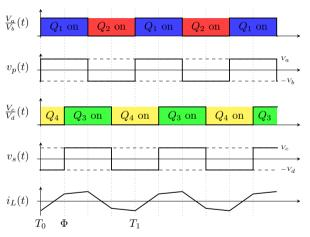
Phase-shift modulation, showing the Mosfet state, Bridge voltages and current through the leakage inductor  $L_r$ .
