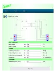
Design tool to calculate the current waveform and power transfer.
