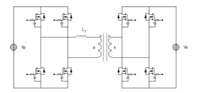
Dual Active Bridge with leakage inductance shown next to the coupled inductors.
