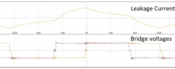
Measurement of full power transfer for  $\varphi=75^\circ$ . From top to bottom: Leakage inductor current[Ch5-Orange, 5A/div,  $4\mu s/div$ ] and primary[Math1-Orange] and secondary[Math2-Purple] transformer voltage[50V/div,  $4\mu s/div$ ].
