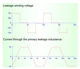
Voltage across and current through the leakage inductor  $L_r$ .
