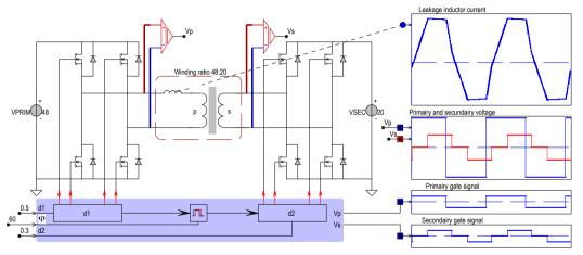
Simulation in Caspoc, of a DAB using two full bridges. The scope show from top to bottom, leakage inductor current, primary and secondary transformer voltages and left and right bridge gate signal.
