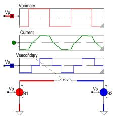
Simplified model in Caspoc, containing the two bridge voltages as controlled voltage sources coupled by only the leakage inductor  $L_r$ .
