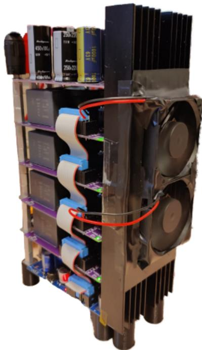
Interleaved bidirectional boost converter PCB
