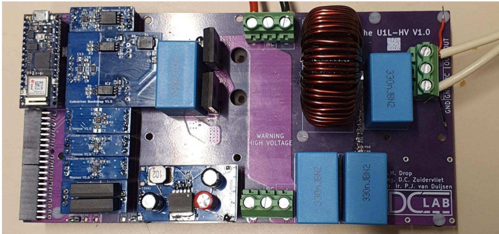
High Voltage Step-Up Converter(Solar Panels)
