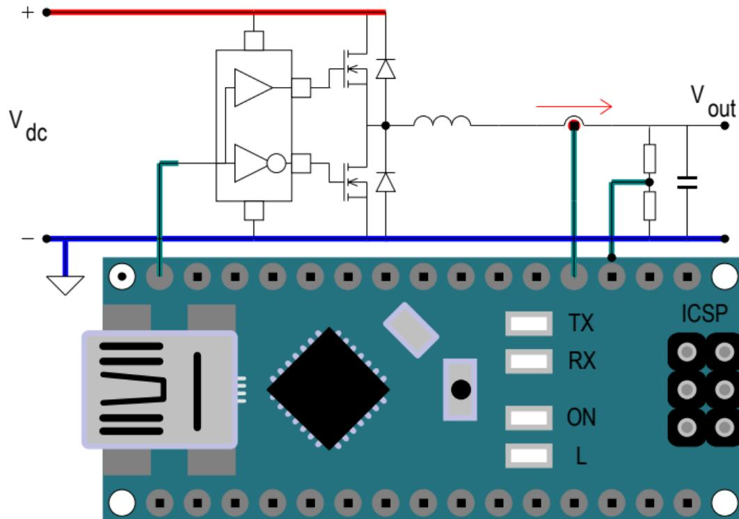
Low Voltage Step down Converter
