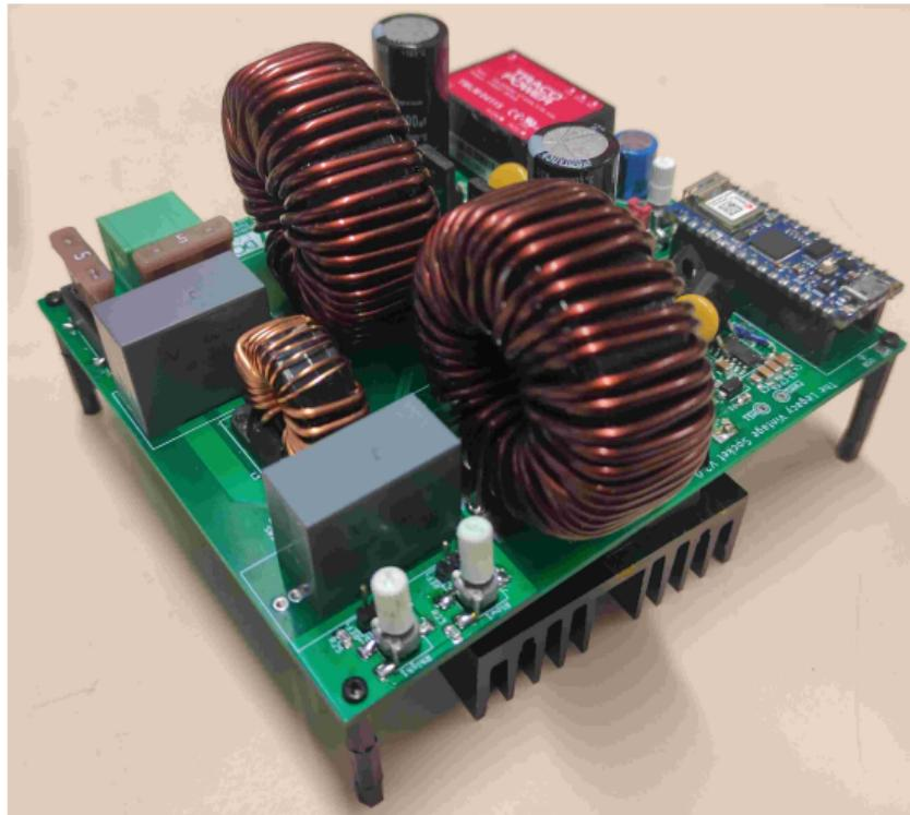
Design, Legacy socket, to create AC230V/50Hz from DC350V.
