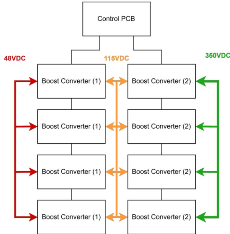
Bidirectional Buck / Boost converter, Interleaved
