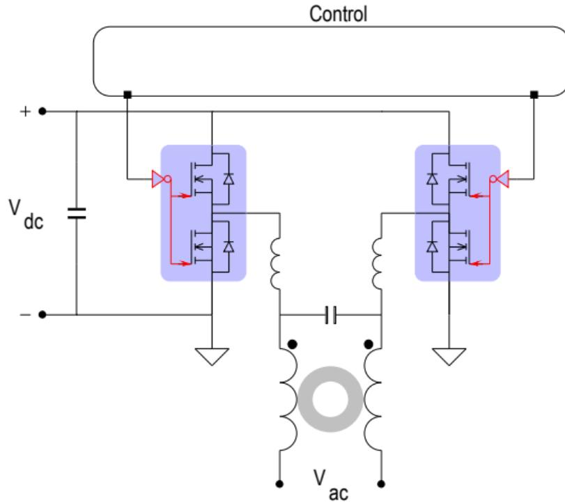
Schematic, Legacy socket, to create AC230V/50Hz from DC350V.
