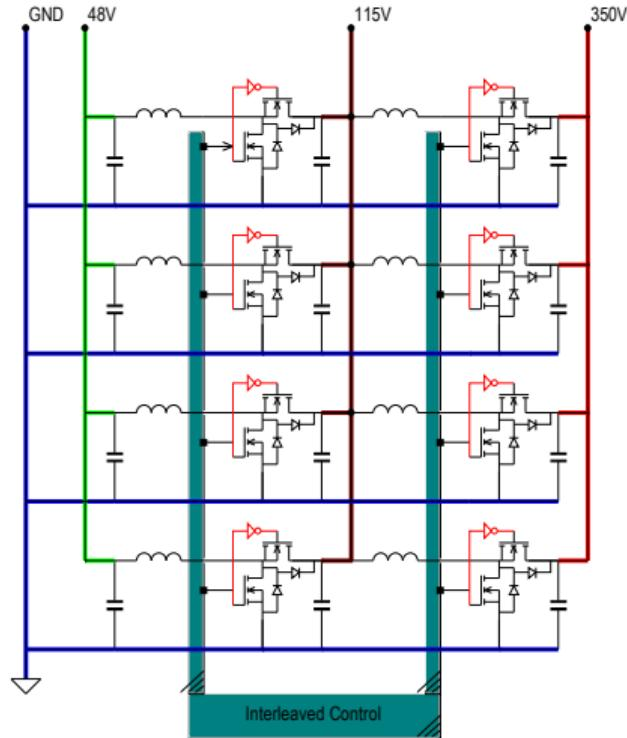
Interleaved bidirectional boost converter Schematic
