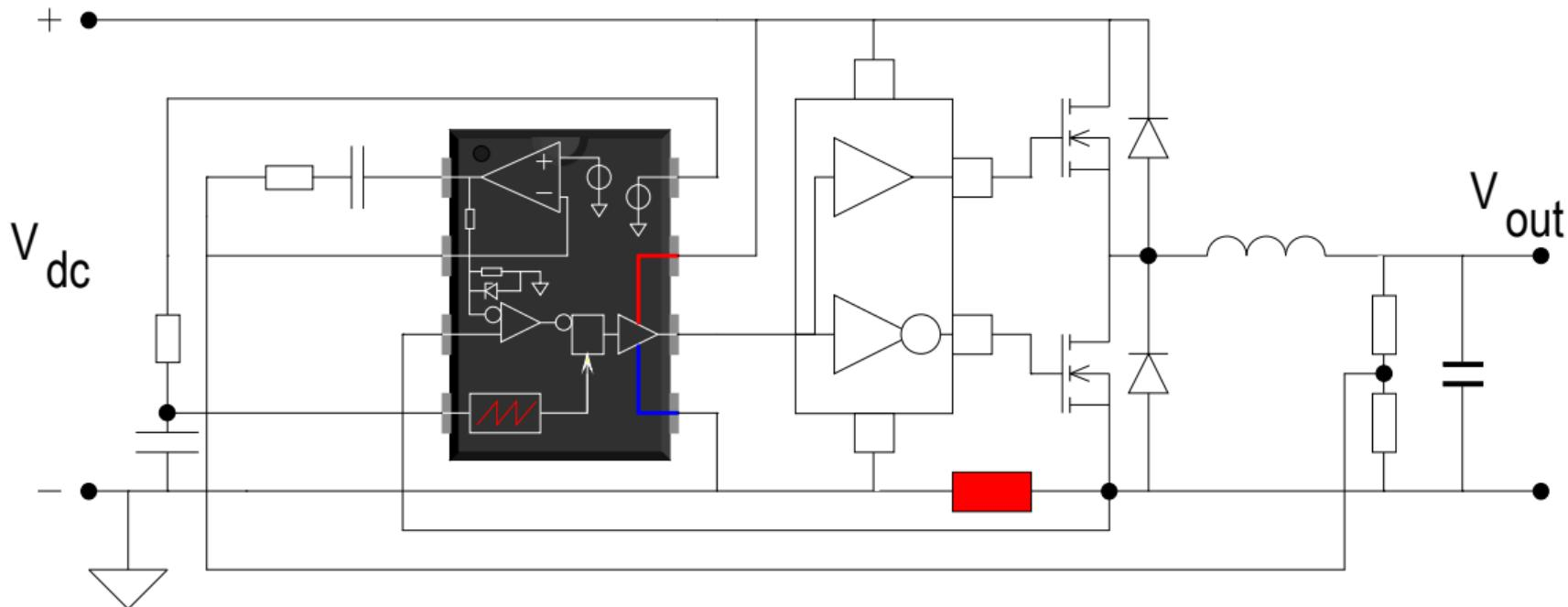
Buck converter with current mode control and floating output.
