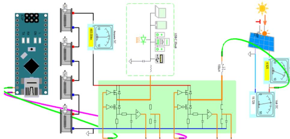
Simulation in Caspoc of droop control and two legs. A solar panel is controlled from leg 1 using a build-in maximum power point tracker, while leg 2 includes the droop characteristic for an USB-C connector feeding multiple devices
