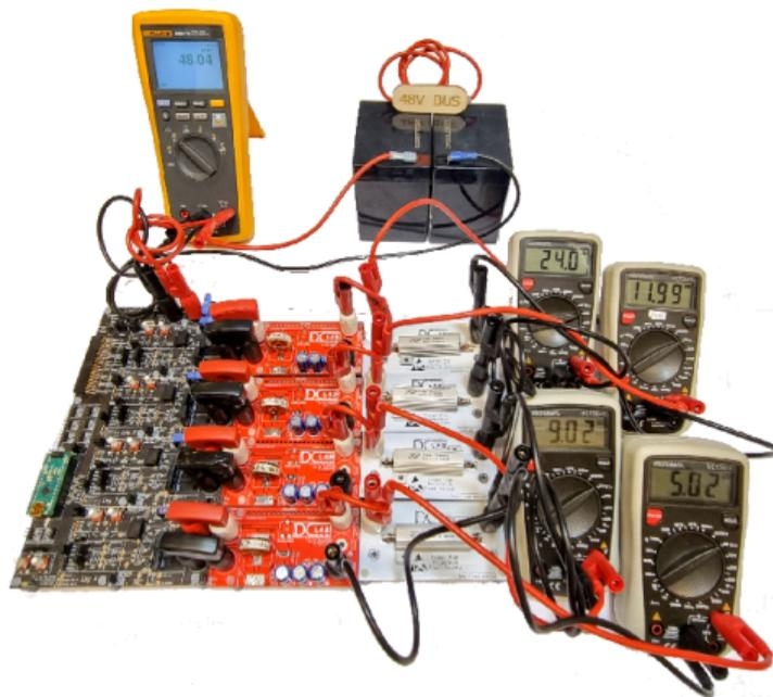
The U4L laboratory setup is connected to a 48Vdc nominal bus. Every leg is connected to a  $10\Omega$  resistive load, creating four nominal voltage levels 5V, 9V, 12V, and 24V.
