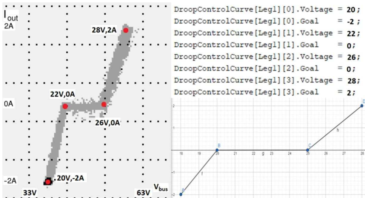
The static droop characteristic of the leg producing 24volt, compared to the implementation of the droop characteristic in the Arduino Nano.
