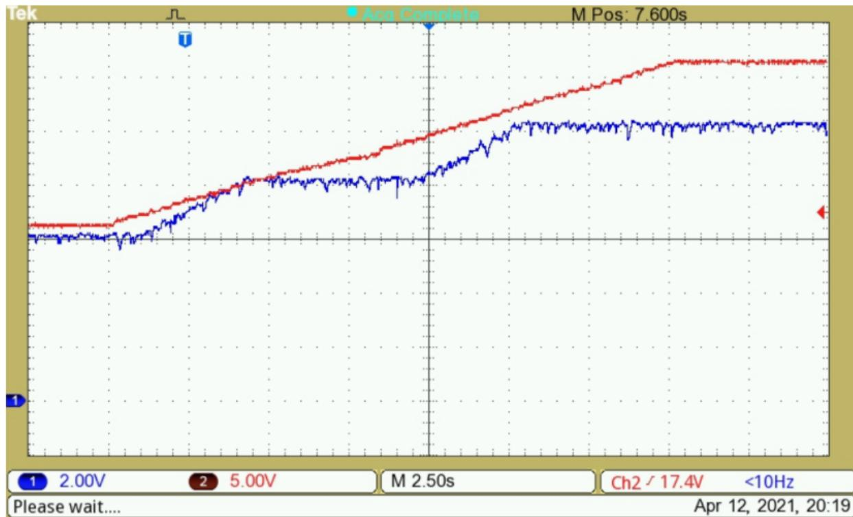
Dynamic behavior, increasing voltage (Red trace) and increasing usage of power (Blue trace).
