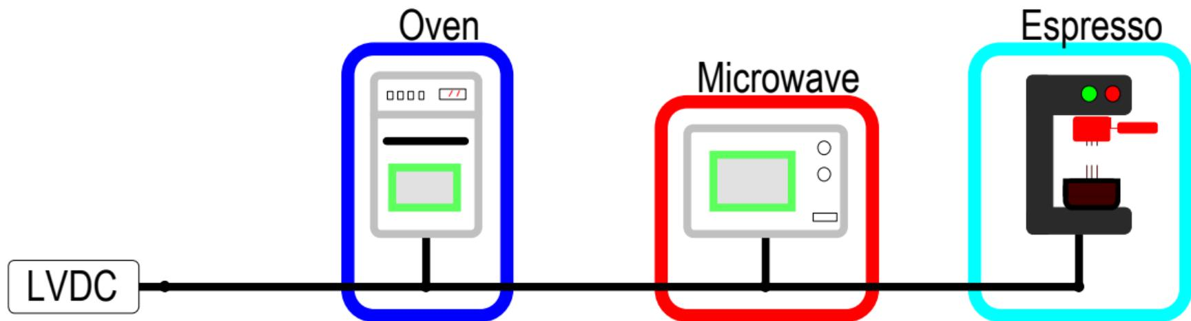
Oven, microwave, and espresso machine connected via a single line to a DC grid.
