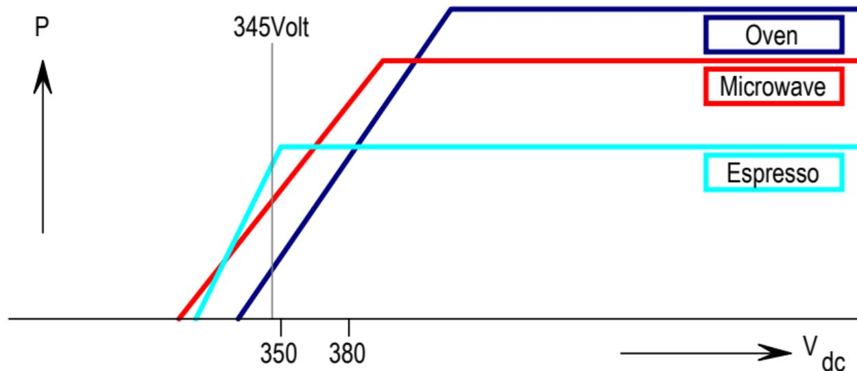
Droop control characteristic per appliance, oven(blue), microwave(red) and espresso machine(lightblue).
