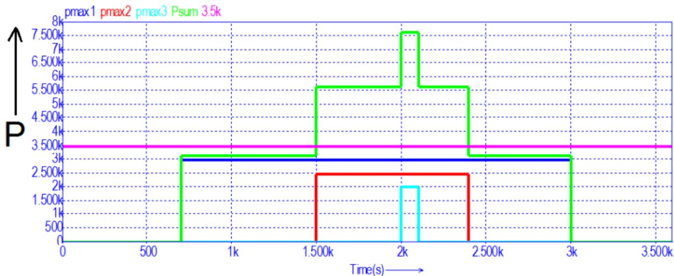
AC Power consumption in Watt(Y-axis) for the oven(blue), microwave(red) and espresso-machine(light blue). Total power consumption(green) is larger than the maximum power consumption allowed by the circuit breaker(magenta).
