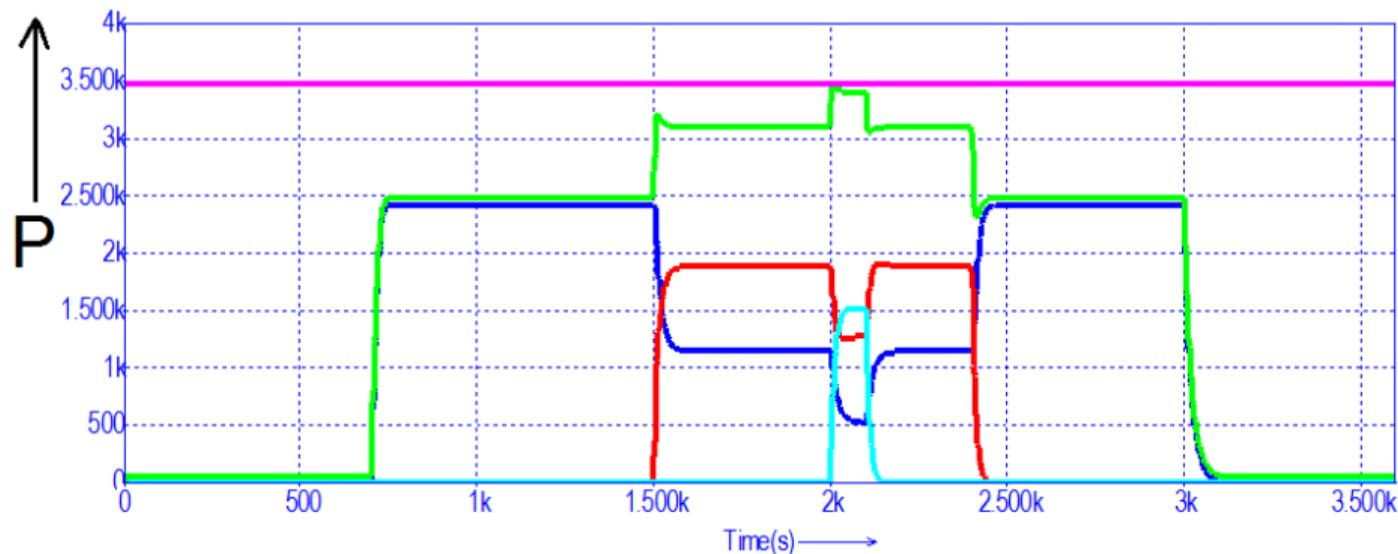
DC Power consumption in Watt(Y-axis) per appliance, oven(blue), microwave(red) and espresso-machine(lightblue), total power consumption(green) below the maximum allowable power consumption limit(magenta).
