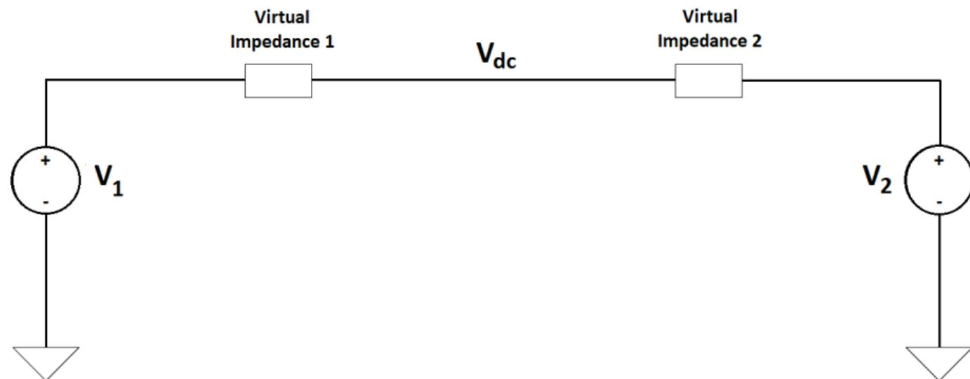
Voltage  $V_{dc}$  depends on the current through the virtual impedance, here represented by two resistors between the two voltage sources  $V_1$  and  $V_2$ .
